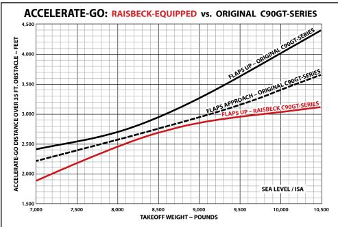
• Increased thrust from our new Swept Blade Props provide large reductions in required airport runway lengths
