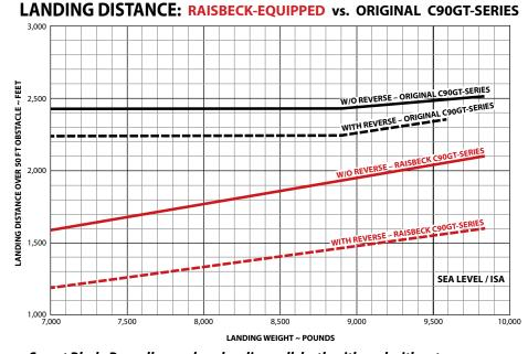
• Swept Blade Propellers reduce landing roll, both with and without prop reverse
