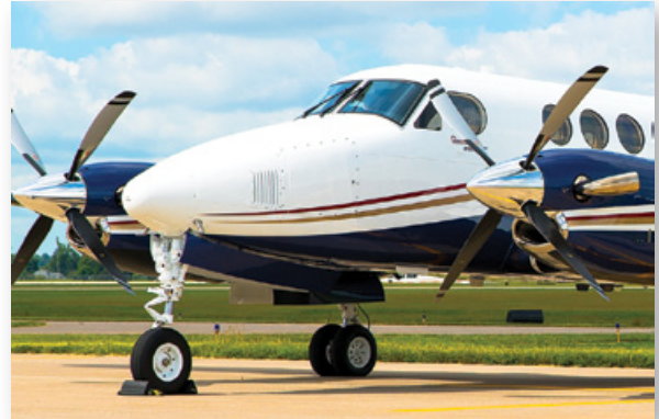
Aluminum 4-Blade Swept Propellers for 250/B200GT/B200/200s Key Benefits: More thrust; less noise; 6-yrs/4,000 hrs TBO
