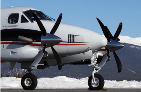
Aluminum 4-Blade Swept Propellers for C90s (all) & E90s Key Benefits: More thrust; less noise; 6-yrs/4,000 hrs TBO
