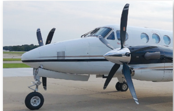
Composite 5-Blade Swept Propellers for 350s Key Benefits: More thrust; less noise; unlimited blade life; 6-yrs/4,000 hrs TBO Available soon for 300s
