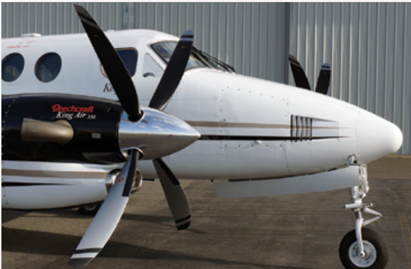
Aluminum 4-Blade Swept Propellers for 350s Key Benefits: More thrust; less noise; 6-yrs/4,000 hrs TBO Available soon for 300s
